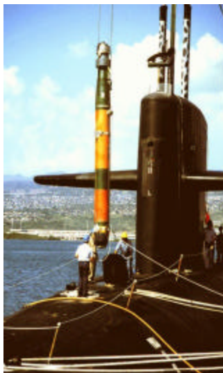
Getting loaded: A Trident sub being armed with a MK 48 torpedo. Loading cruise missiles is the next task for four refurbished Tridents. Photo: http://www.fas.org/nuke/guide/usa/slbm/731-p05.jpg
